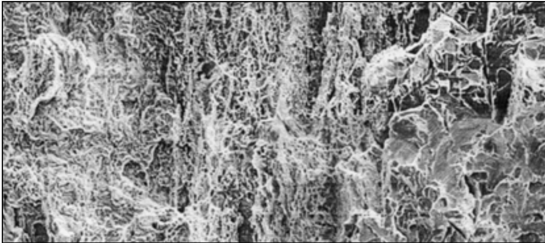
Fig. 3. Fracture surface in powder iron [11] obtained under the conditions of static loading at 20°C and dynamic final breakage at -196°C. × 100.
