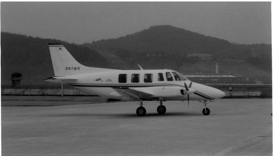
Figure 1. All-composites aircraft (courtesy: Korea Aerospace Research Institute).
