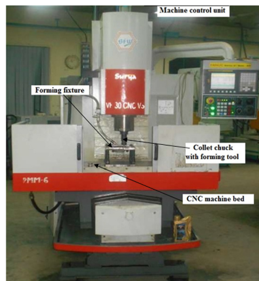
Fig. 1 – Experimental setup for single point incremental forming process on CNC milling machine.
