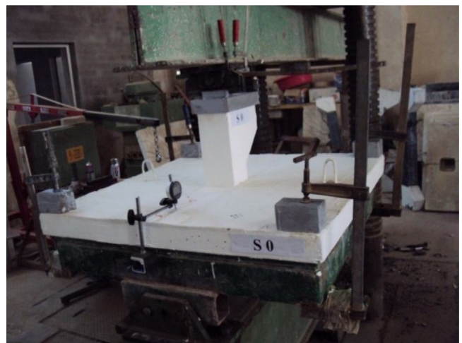
Fig. 7 – Loading frame and a typical slab.
