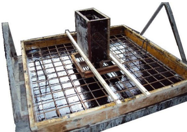
Fig. 6 – Shearhead position in the slab.
