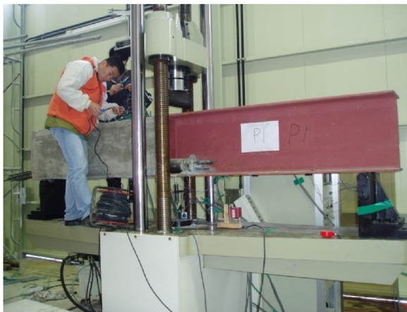
Fig. 8 – Three-point bending test of hybrid girder test member.
