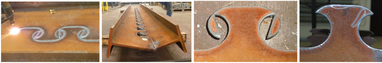
Fig. 2 – Consecutive stages of obtaining steel T-beams with MCL connectors.
