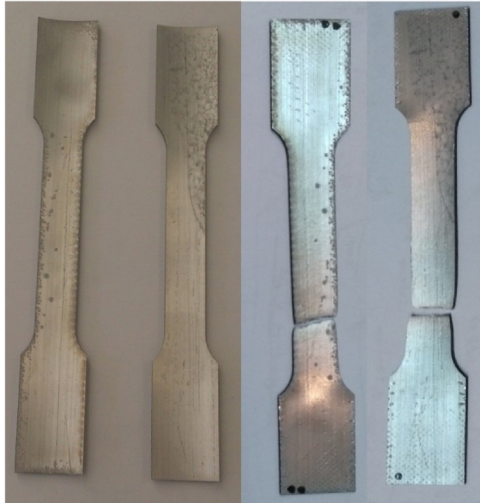
Fig. 1 – Tension test samples before (left) and after (right) test.
