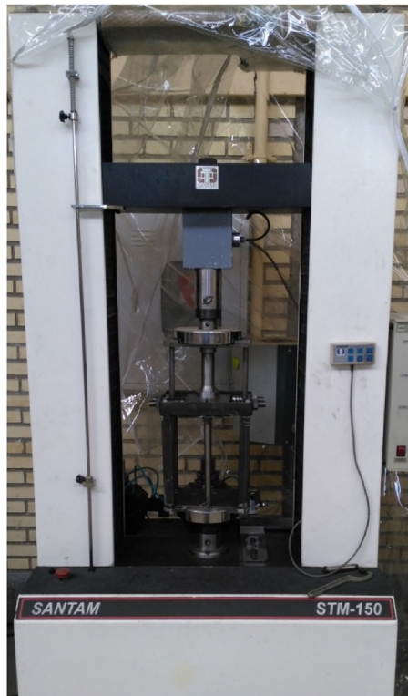
Fig. 5 – Santam apparatus with installed fixture.
