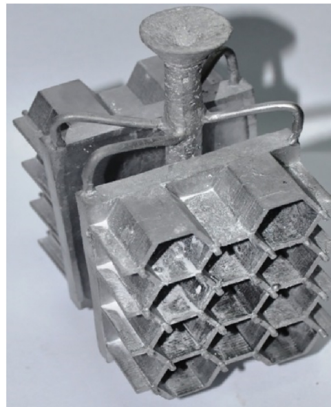
Fig. 3 – Honeycomb structure castings with gating.
