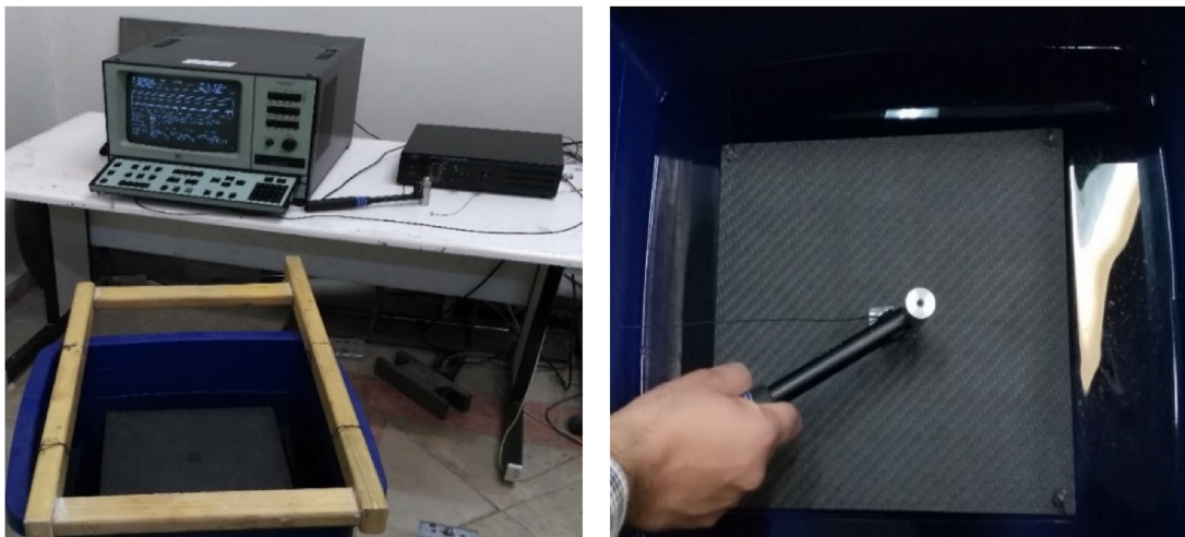
Fig. 10 – Experimental setup for modal testing.
