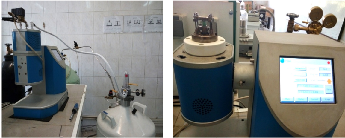
Fig. 2 – The DMA test setups.
