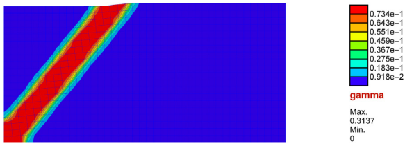
Fig. 13 – Deformed mesh (mesh1) for conductive, plane strain conditions with BDP plasticity, imperfection 20% of \sigma_{y0} , \phi = 15^\circ , k = 100 \text{ J/(s K m)} , ideal plasticity.
