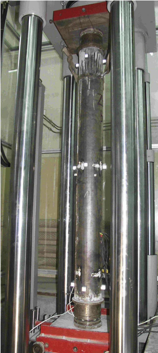
Fig. 2 – The hydraulic press with the column prepared for the test.
