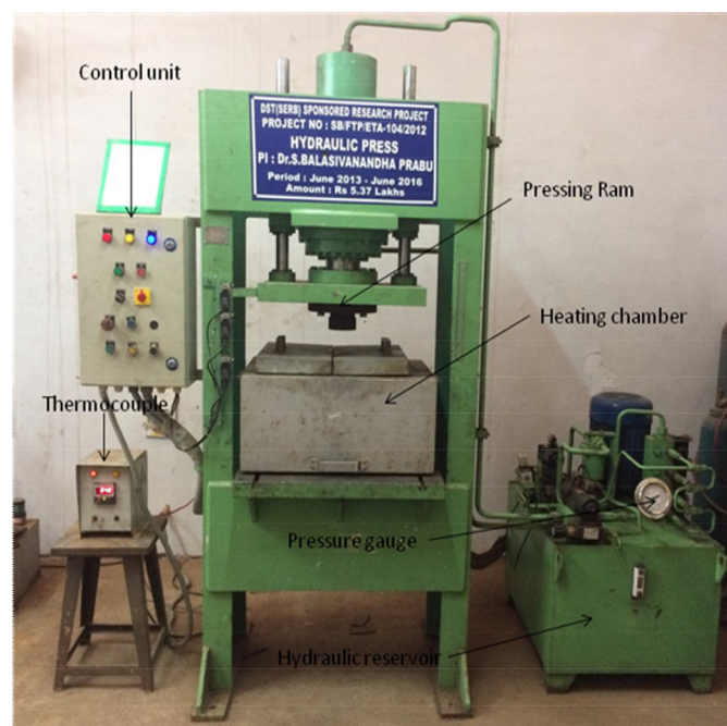
Fig. 2 – Schematic view of hydraulic press with heating chamber mounted and thermocouple with a PID controller.
