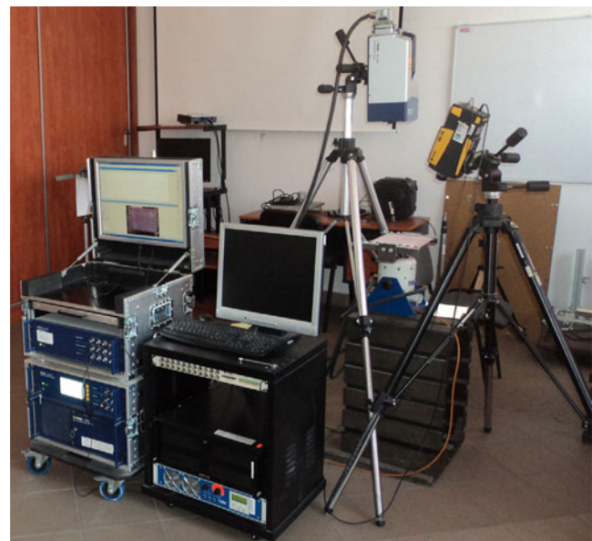
Fig. 7 – Experimental setup of vibration-based non-destructive tests.
