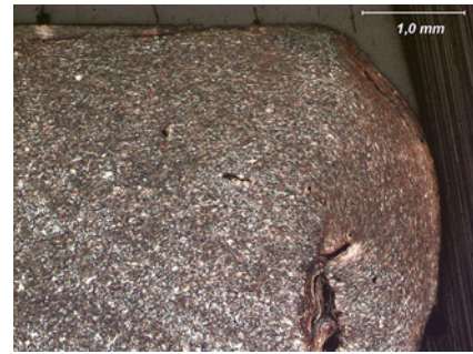
Fig. 6 – A microscopic image of the structural alterations and damages. Elongated visible (light) parts are ferrite separations. Magn. 25x, etched 3% \text{HNO}_3 , light microscopy.
