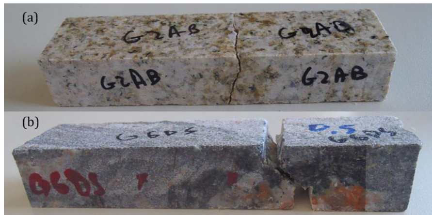
Fig. 4 – Typical specimens after fracture (a) bending, (b) shear.
