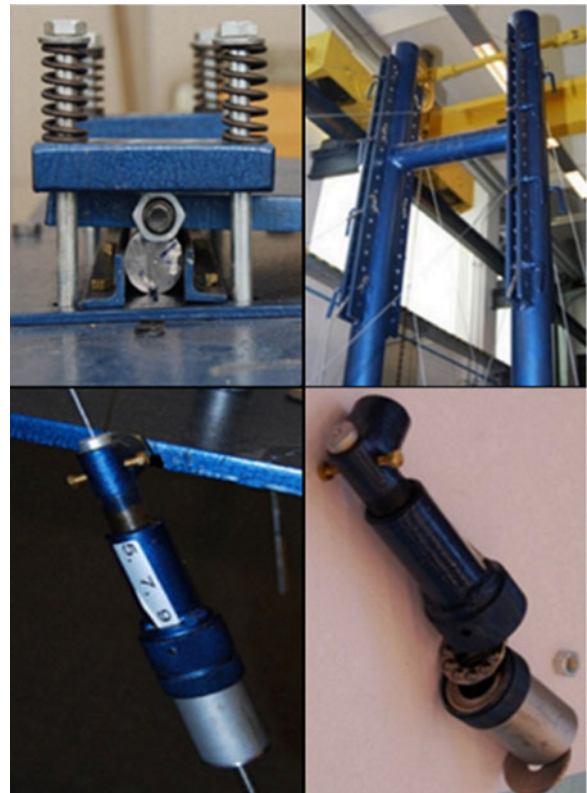
Fig. 3 – Tension regulator and construction details.
