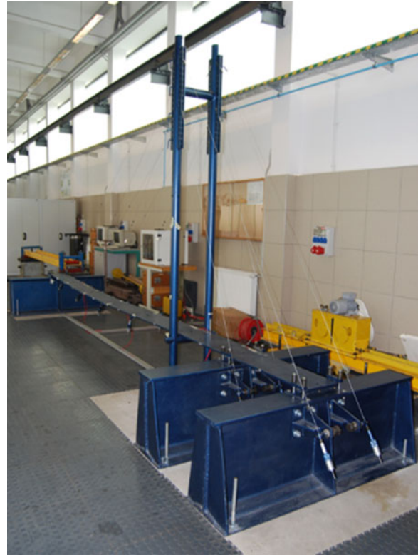
Fig. 2 – The model of the footbridge in laboratory, the Institute of Civil Engineering.
