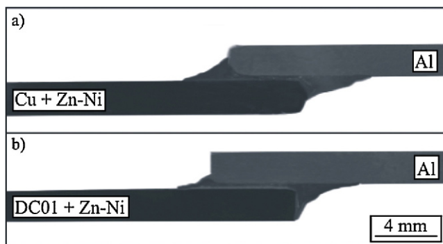
Fig. 4 – Soldered overlap joints: Al-Cu-ETP + Zn-Ni layer (a) and Al-DC01 + Zn-Ni layer (b) made with L-ZnAl4 solder.
