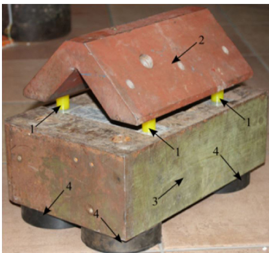
Fig. 3 – Test rig: 1 – tested specimens; 2 – vibrating mass; 3 – seismic mass, 4 – damping washers.
