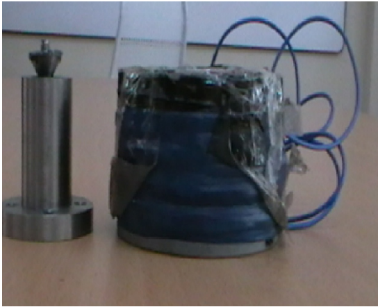
Fig. 6 – Dissembled view of the MR fluid system.
