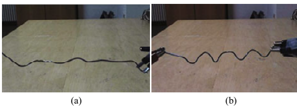
Fig. 12 Proof of concept about SMA bio-tendril FC pulling phase [55] : (a) Starting; (b) final configuration.
