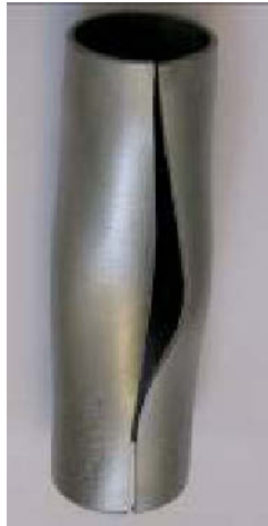
Fig. 10. Panel deformation ( L = 100 mm, \theta = 355^\circ )
