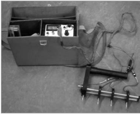
Fig. 5. Concrete resistivity measurement system (CNS Equipment)
