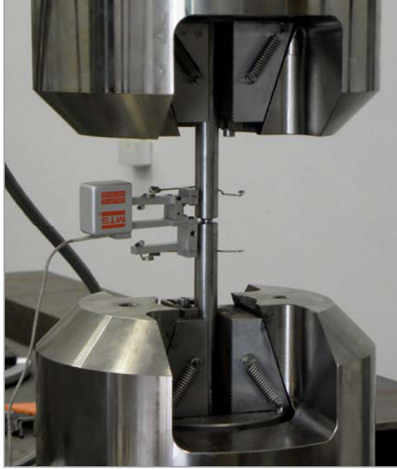
Fig. 7. View of a ring-notched round specimen subjected to tension in a complex stress state
