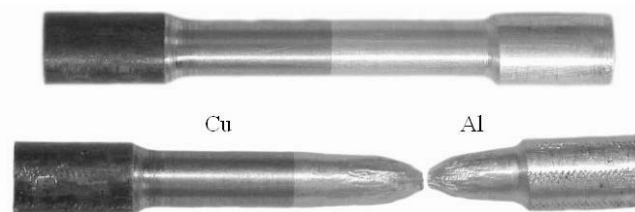
Fig. 3. A view of an Al-Cu sample before and after tensile test [4]
