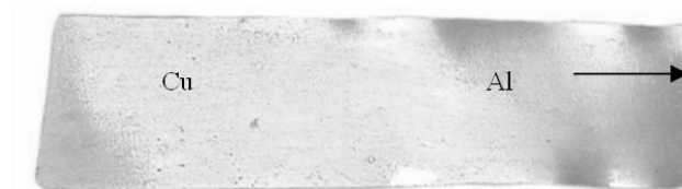
Fig. 6. Al-Cu sample after longitudinal rolling with a small cold work in each pass [4]
