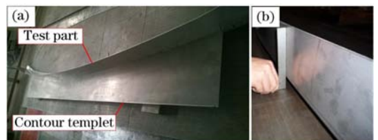
Fig. 14 Test part with high contour accuracy (a) and little cross section distortion (b)
