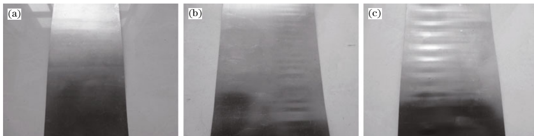
Fig. 6 Test results for different taper angles of 0.0013 (a), 0.0023 (b) and 0.0033 (c)
