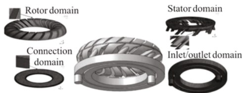
Fig.8 Mesh optimization of the computational domain
