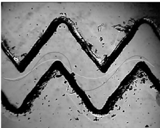
Fig.7 Particle trajectory at the Reynolds number of 94
