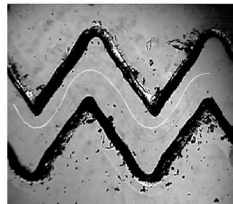
(a) Particle trajectory at the inlet of the labyrinth channel
