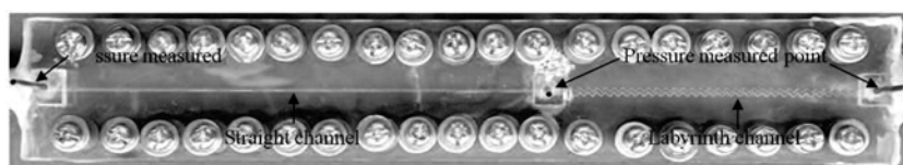
Fig.2 The emitter channel model used for testing
