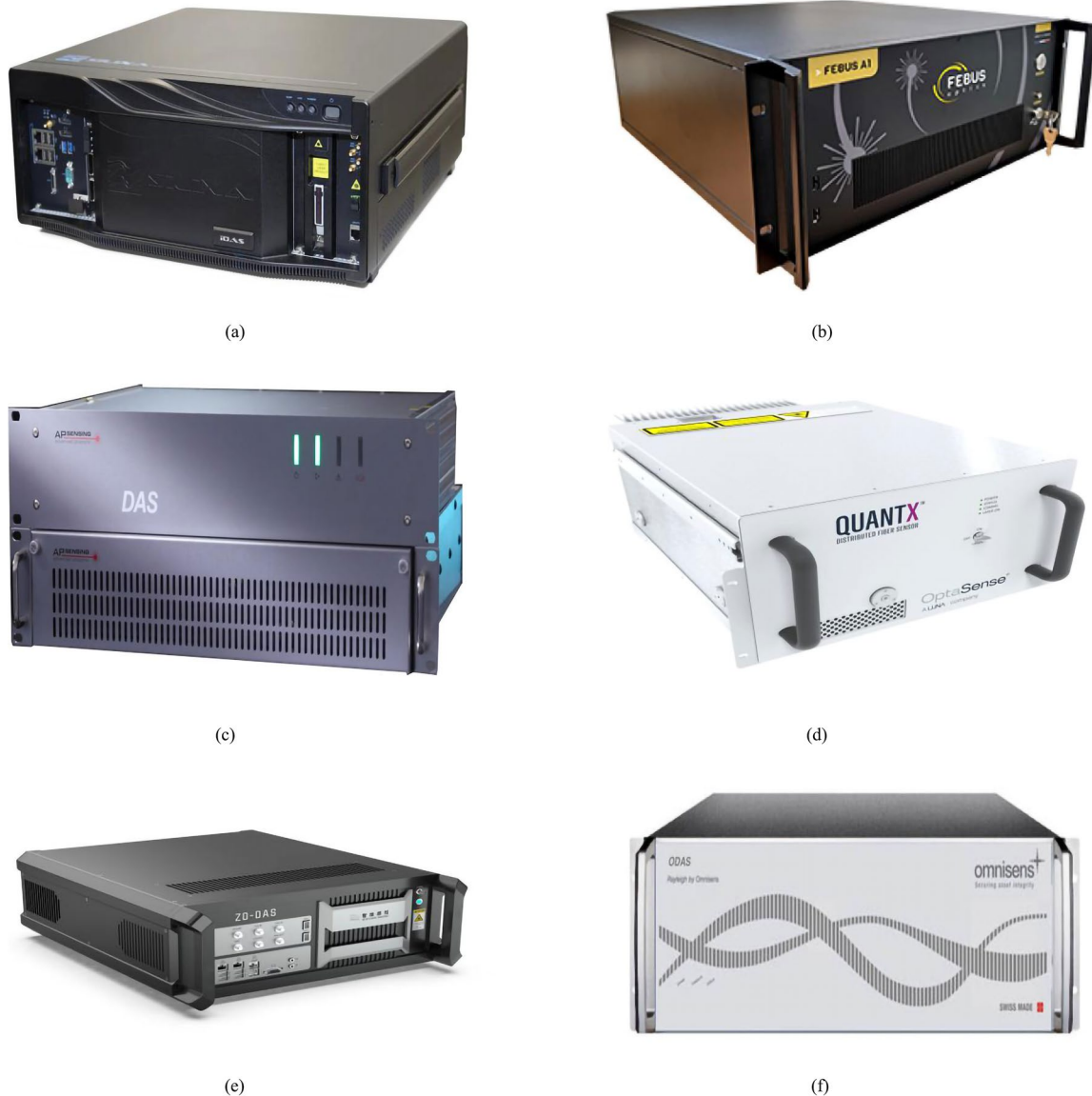
Fig. 1 Distributed acoustic sensing (DAS) equipment diagram. a IDAS; b FEBUS A1-R; c AP SENSING DAS; d OptaSense QuantX DAS; e USTC ZD-DAS; f Omnisens DITEST
