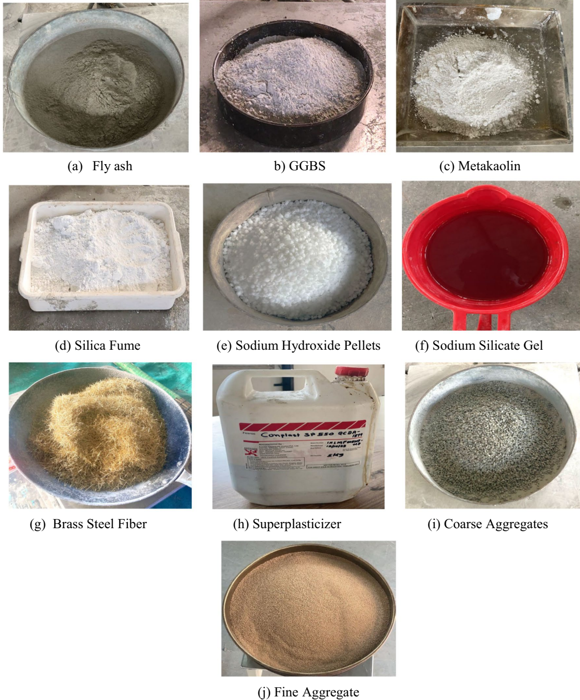
Fig. 1 Photographs of materials used in the experiment. a Fly ash. b GGBS. c Metakaolin. d Silica Fume. e Sodium Hydroxide Pellets. f Sodium Silicate Gel. g Brass Steel Fiber. h Superplasticizer. i Coarse Aggregates. j Fine Aggregate
