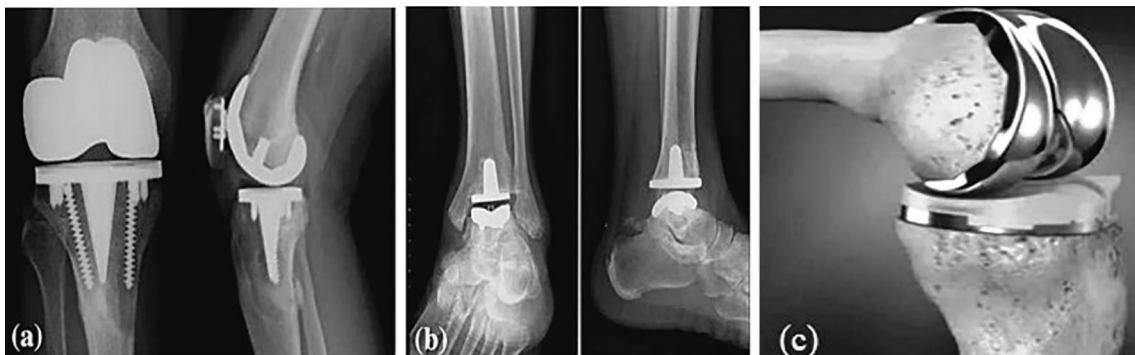
Fig. 57 Stainless steel implants in a knee and b ankle. c Knee replacement made from CoCrMo alloy [165]
