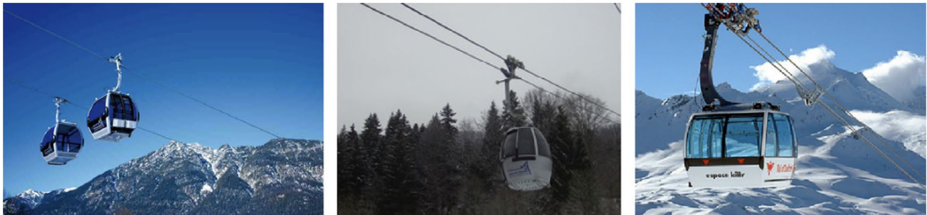
Fig. 49 Mono-, bi- and tri-cable ropeways [145]
