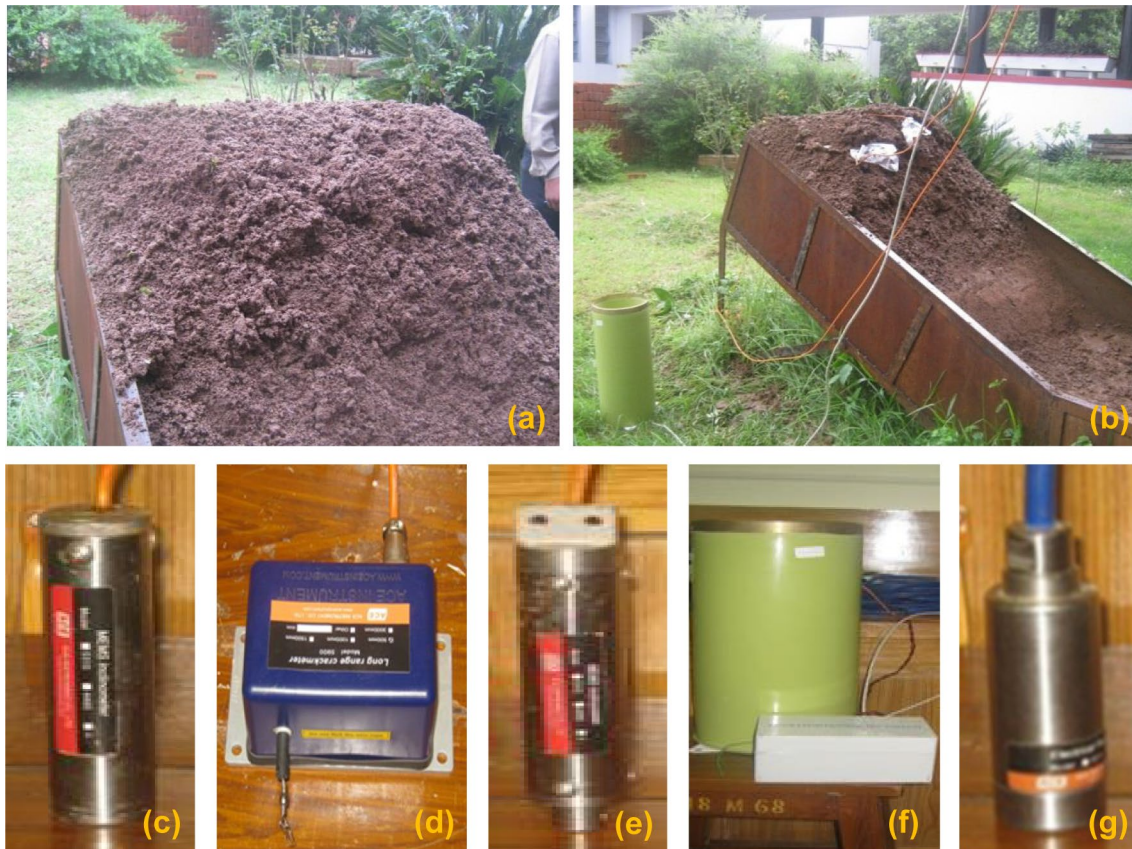
Fig. 5 View of test bed and geosensors utilized in the laboratory experiment for monitoring landslides: a test bed, b sensor connections in the test bed, c tiltmeter, d crackmeter, e in-place inclinometer, f rain gauge, and g piezometer
