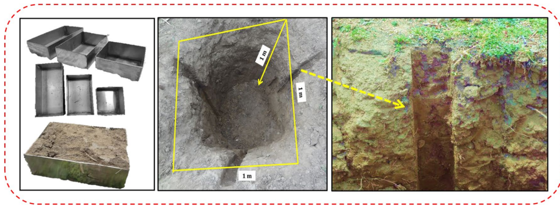
Fig. 2 Pit-based depth-incremental procedure followed for soil sampling
