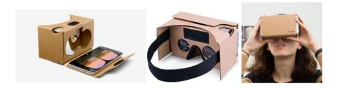
Using the Cardboard results in an impressive VR experience. The Cardboard's VR meets all Chalmers' criteria for full-blown VR: it is computer-generated because it depends on the phone's computations. It is interactive because the phone's rotation sensors, and magnet, allow one to look around the virtual world and interact with it respectively. And it is immersive because the experience elicits a sense of being present in a virtual world.<sup>8</sup>
