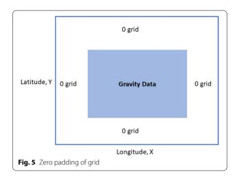
Fourier Transformation, which is required for computing residual gravity anomalies. The assessment and evaluation of the computed residual sea surface height,  $h_{residual}$ , are implemented in these equations.
