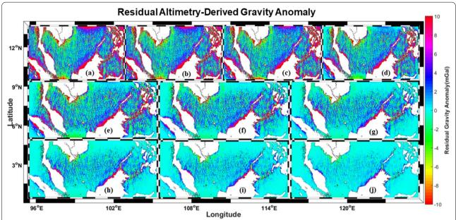
**Fig. 7** Residual gravity anomaly distributions from tapering window width 5 (**a**), tapering window width 10 (**b**), tapering window width 20 (**c**), tapering window width 50 (**d**), tapering window width 70 (**e**), tapering window width 100 (**f**), tapering window width 125 (**g**), tapering window width 150 (**h**), tapering window width 170 (**i**) and tapering window width 200 (**j**)
