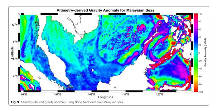
After performing the cross-validation procedure, the RMSE value decreased by approximately  $\pm\,0.0524$  mGal to 0.0845 mGal. Thus, the final output provides the altimetry-derived gravity anomaly model over Malaysian seas with good accuracy based on RMSE values of  $\pm\,4.2472$  mGal to  $\pm\,6.0202$  mGal.
