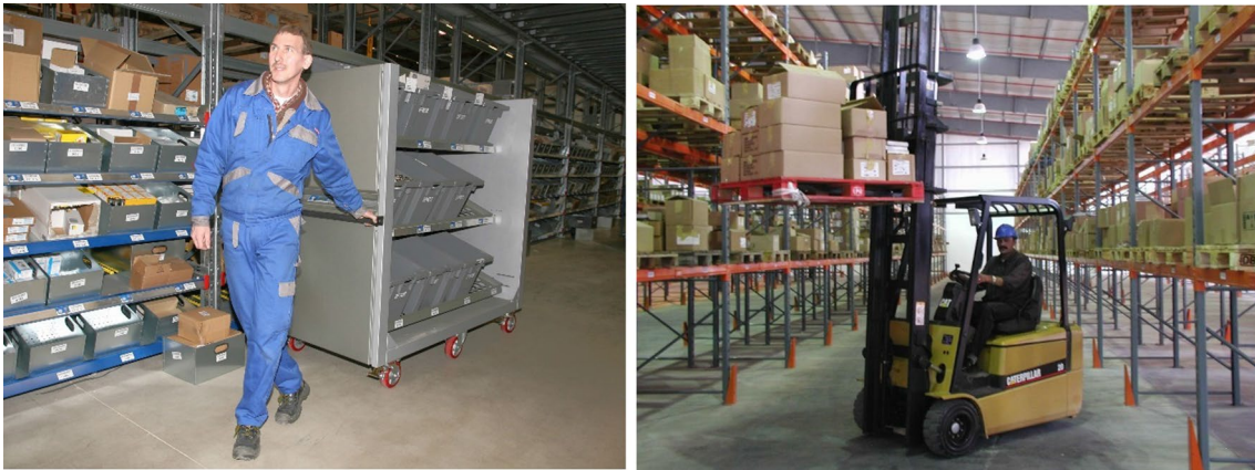
Fig. 1 Examples of equipment used for material handling; a human puller, i.e., cart carrying bins of parts (left) and a forklift moving heavy materials (right). Credits: (Left) KBS Industrieelektronik GmbH, “Pick-by-Light Kommissionierfahrzeug mit neun Zielbehältern”, July 1 2010, Used under Creative Commons Attribution-Share Alike 3.0 Unported license, Online at https://commons.wikimedia.org/wiki/File:Pick-by-Light_Kommissionierfahrzeug_PickTerm_Cart.jpg , Accessed July 21 2021. (Right) Bakker, J. J., “Sonneborn Refined Products BV Spaarndamseweg 466”, June 12 2009, Used under Creative Commons Attribution 2.0 Generic license, Online at https://commons.wikimedia.org/wiki/File:Forklifter_at_Sonneborn.jpg , Accessed July 18 2021
