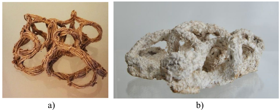
Fig. 3 a) hemp strings after soaking and bringing into form, b) sample after drying; ©IBK2, Student: Tian Mi / University of Stuttgart
