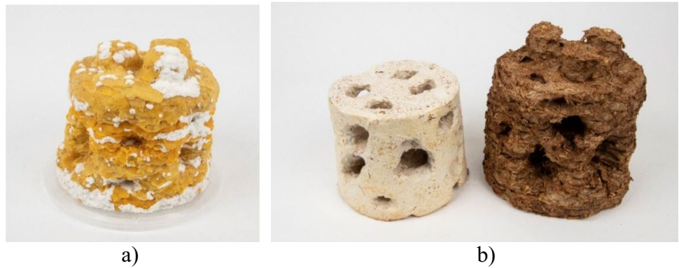
Fig. 2 a) Test B sample after growth period, b) Test A and Test B after oven drying; ©IBK2, Student: Daniel Pauli / University of Stuttgart
