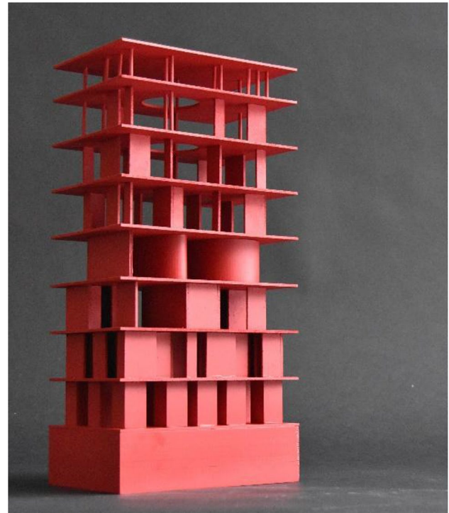
Fig. 12 This model employs a distinct box-like strategy in the lower stories. AHO/Multistory Building (MSB), 2018. Project and model by; Are Hagen, Kaja Strand Ellingsen. Photo; Joar Tjetland
