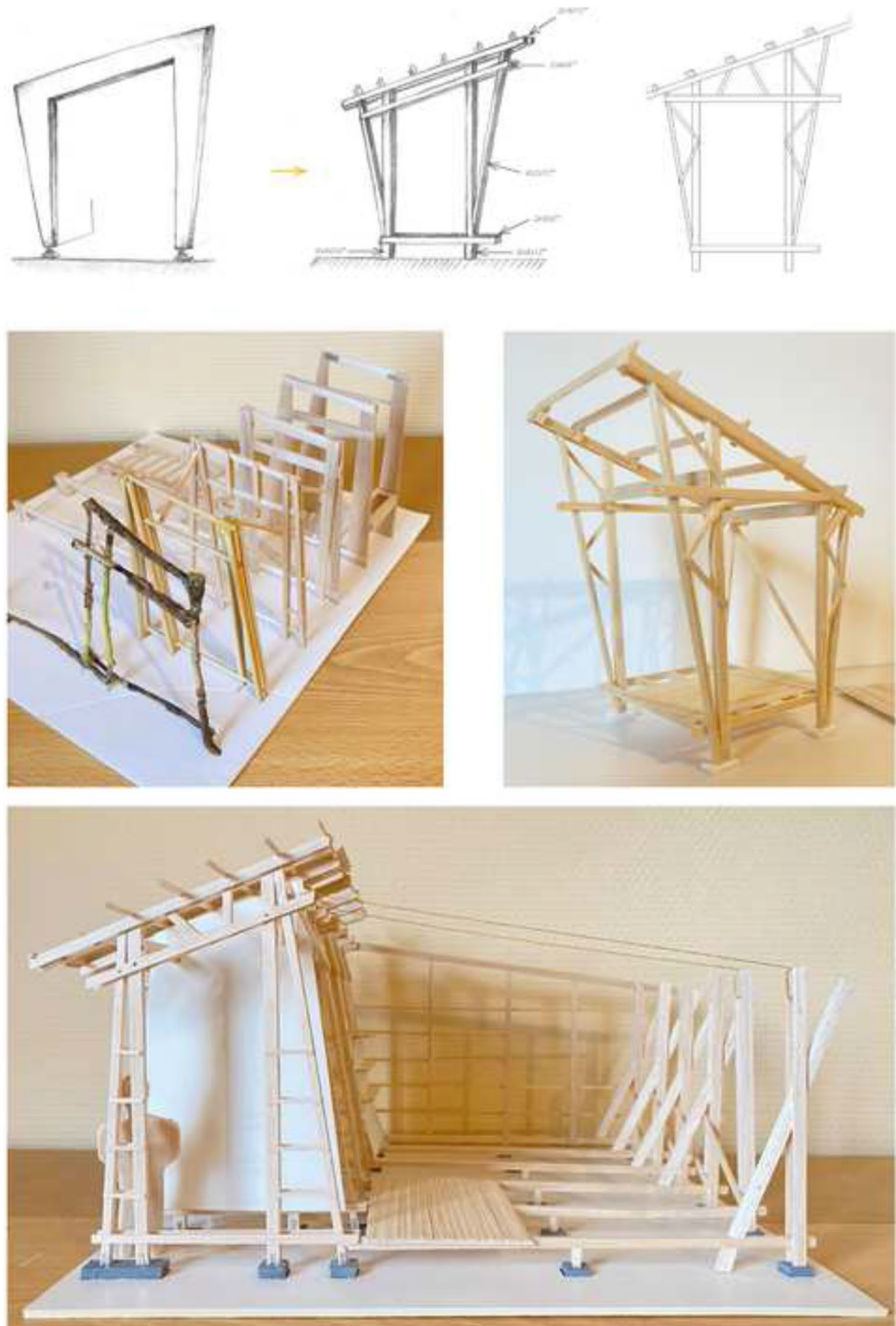
Fig. 5 Example Structural Typology . (Above and middle) The student's interest in local Philippine houses leads to structural and constructive explorations of wooden portal frames. (Below) The model of the final design outcome. (Courtesy of Stephanie Alatraca)
