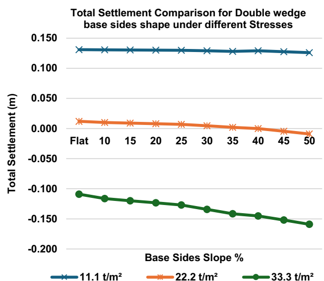
Fig. 17 Relationship between double wedge base sides slope and total settlement curve for applied stresses of 11.1, 22.2, 33.3 t/m 2
