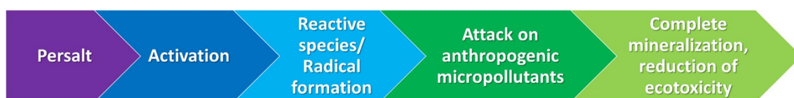
Fig. 2 General process of persalt-induced anthropogenic micropollutant removal
