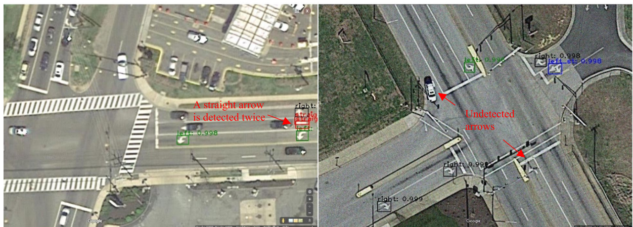
(b) Incorrectly detected lane-use arrows
