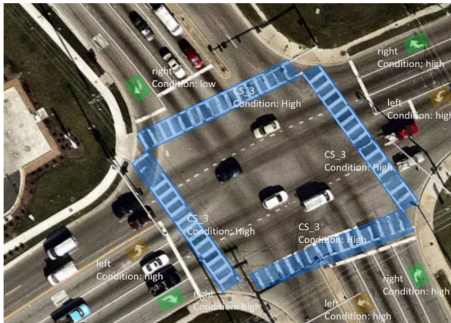
Fig. 2 Overall annotated image with land-use arrows, crosswalks, and degradation conditions labeled
