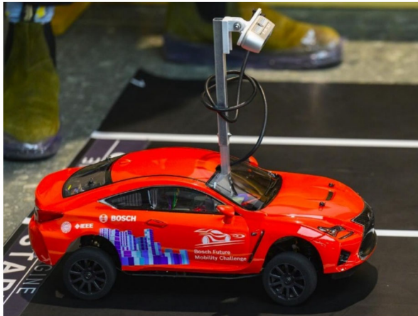
Figure 1 1:10 scale model car including sensors, compute platforms, and actuators
