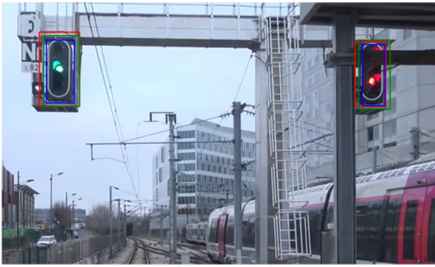
Fig. 2 Bounding boxes as predicted by the ML predictor (blue), their conformalized version with additive scores (green) and the ground truth (red). Example of images used in conformalization and testing, cropped for readability
