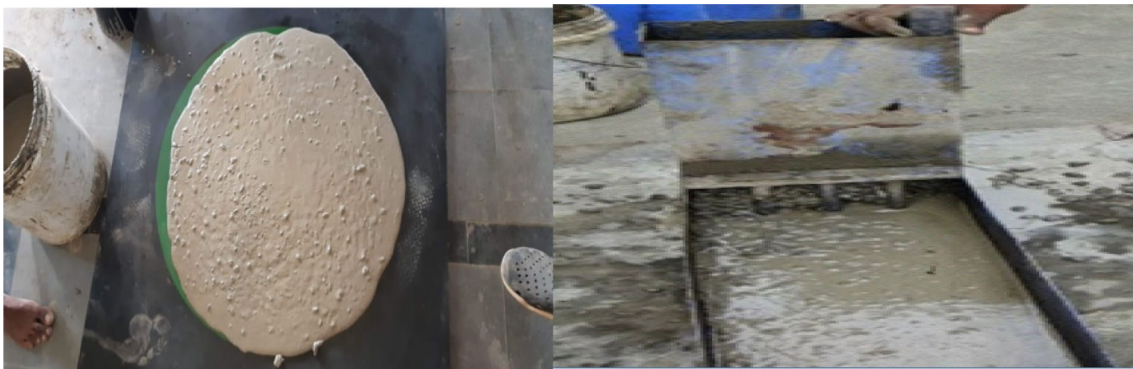
Fig. 2 Slump flow and L-box
