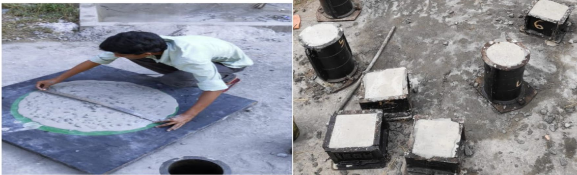
Fig. 1 Slump flow tests and placements of concrete in the specimen
