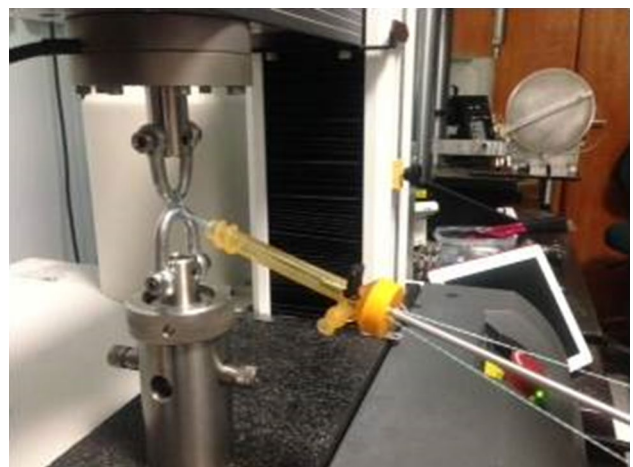
Fig. 3 Knot tying process using an 8.4 mm cannula assisted with a single-hole knot pusher
