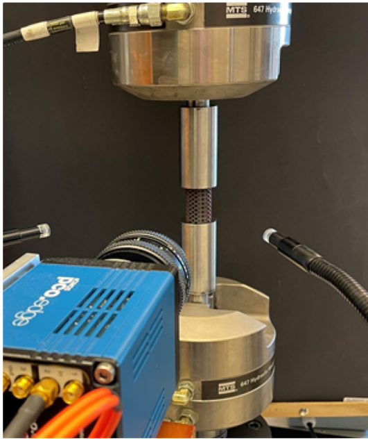
Fig. 5 Experimental setup with one of the porous samples inserted in between two hydraulic grips with adjustable clamping force
