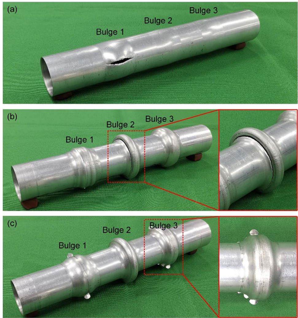
Fig. 24 Forming defects in hydroforming of the tubular component with three bulges: a splitting on the straight tube blank; b splitting on the wrinkled tube blank; c undercut on the wrinkled tube blank
