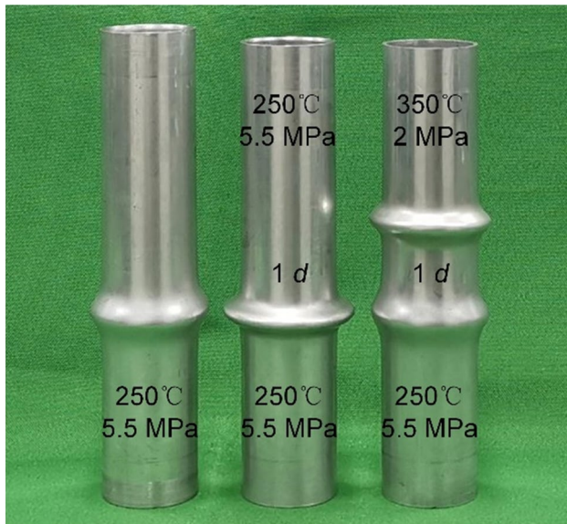
Fig. 16 Wrinkled tube specimens with two wrinkles obtained under different internal pressures
