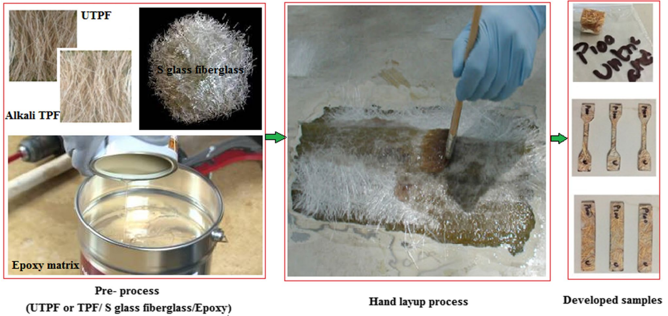
Fig. 1 Details fabrication layout and its test samples
