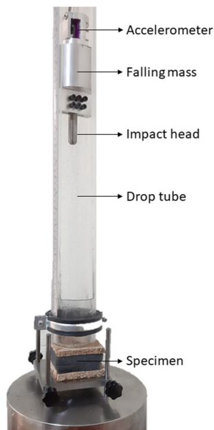
Fig. 3 Experimental setup for deceleration tests
